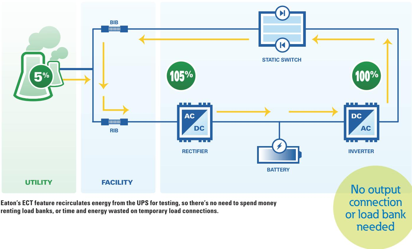
Eaton's ECT feature recirculates energy from the UPS for testing, so there's no need to spend money renting load banks, or time and energy wasted on temporary load connections.
