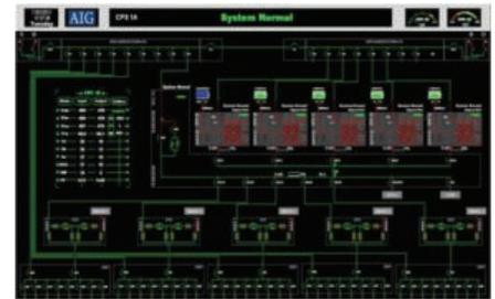
Eaton also offers a flexible system interface configuration (10 inches to more than 40 inches). This LCD monitor is a full representation of the one-line with metering, status, upstream and downstream distribution, and even weather reporting which can control the UPS.
