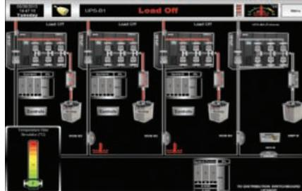
Eaton provides a fully automated SCADA solution that monitors equipment for failures of switchgear bus, cable terminations/joints, bus duct and transformers. This specific system uses IR SCADA monitoring to provide 7x24 continuous monitoring of equipment health as well as predictive failures of buss connections.
