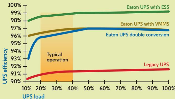
Efficiency generally dips as load levels decrease. However, ESS technology operates at 99 percent efficiency even at low-load levels, providing you with real energy savings.
